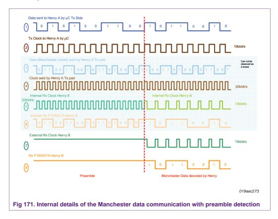
Traces 1 and 2 represent the data and the clock that the microcontroller sends to the OL2381 A (transmitter). The microcontroller sends 0x14C preamble. This data is not Manchester encoded. EncCoding is performed within the OL2381 A. Traces 3 and 4 show the data and clock that the OL2381 A sends after Manchester encoding. After encoding, the OL2381 A sends 0x665A5 "in the air".
