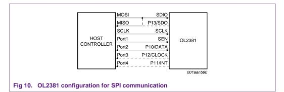
Bits SEP\_TX\_LINES and SEP\_RX\_OUT in register PORTCON2 should be set to logic 00 for a SPI data communication. This is shown in Figure 11.
