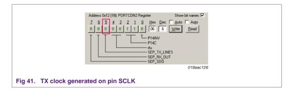
To generate TX clock on pin SCLK or P12/CLOCK, registers PORTCON1 and PORTCON2 must be configured (see Figure 41 and Figure 42).
