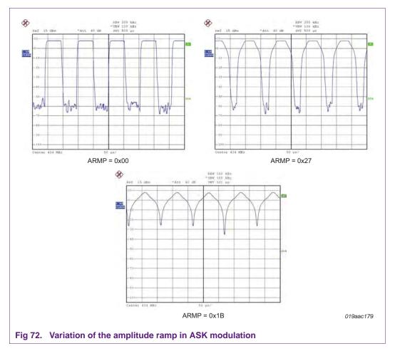
It is important to keep in mind that the value of the amplitude ramp should not be too high. Otherwise, the signal will not have time to reach the low level. Figure 72 shows the ARMP is set to 0x1B ( $27 \times 16$  MHz clock cycles). An optimum amplitude ramp is achieved when the time between the low and high level is 1/3 of the total time period as shown in with Figure 72 ARMP= 0x27.
