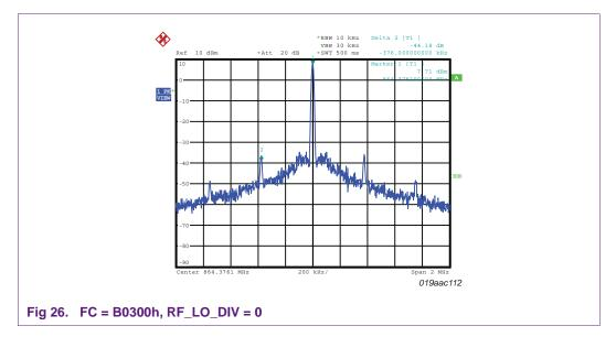
The influence of flag Double\_SD\_Result to the spurious emission is small. If the flag is set, the output signal will show an increased phase noise. Avoid configuring the OL2381 to FSK in transmit mode if the flag is set.
