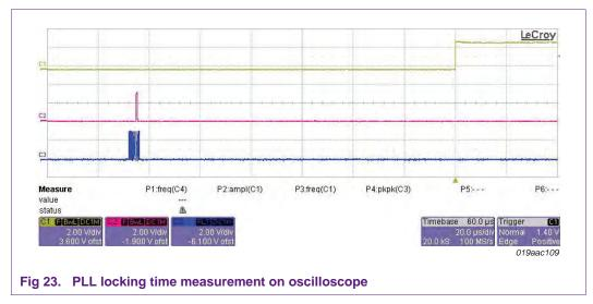
In Figure 23, the yellow trace is the LO\_RDY flag signal at pin P11/INT, the red trace is the write command data on SPI line SDIO, and the blue trace is the SPI clock measured on pin SCLK. PLL locking time is close to 120  $\mu$ s.
