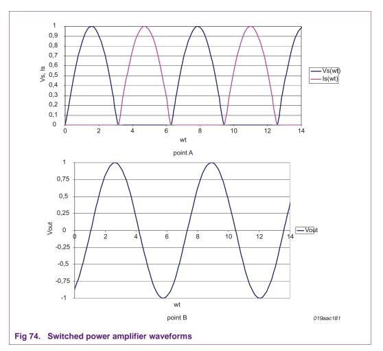
The impedance of a switched PA is modeled by a switch in parallel with a capacitor. Depending on the state of the switch, the impedance changes, and therefore the actual impedance is a linearization around the operation point given by the matching network. The procedure to calculate the matching is derived from the resonant conditions for the class E operation and is explained in <u>Section 6.6.2</u>.
