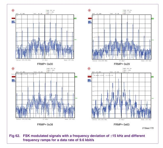
Figure 62 and Figure 63 show the effects of the FRMP on the signal in frequency and time domain with a frequency deviation of  $\pm 15$  kHz and a data rate of 9.6 kbit/s.
