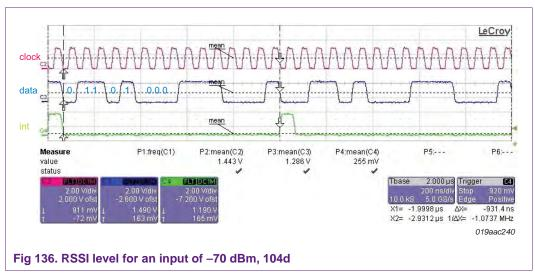
Figure 137, Figure 138, and Figure 139 show an example of how the RSSI level classification can be used in a real application. System design registers LOWERRSSITH and UPPERRSSITH (address: 0x26 and 0x25) are set to 100d and 120d; see Figure 116 on page 87.
