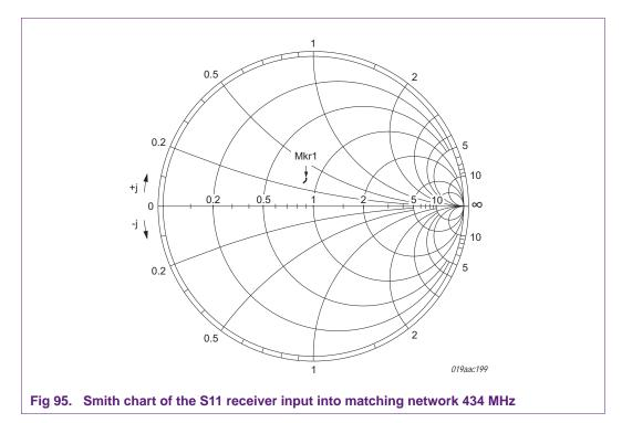
The receiver matching is close to 50  $\Omega$ , the best achievable with standard available values for passive components (L, C) on the market. The different values of receive matching for different frequencies are presented in Figure 95 and Figure 96.
