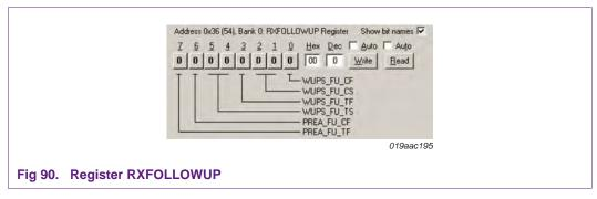
This register determines OL2381's action after successful (or unsuccessful) WUPS and/or preamble when initiated from a polling timer event or by a receive command. If a failed WUPS or preamble detection occurs, the OL2381 can go in to power-down or stop state. Only if the receive mode is activated from a polling timer event, an interrupt can be generated as shown in Figure 91.
