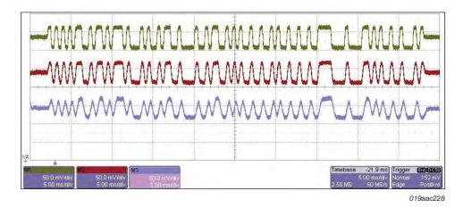
Fig 124. Baseband filter output (baseband filter comparison)
