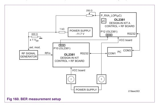
Two OL2381 design-in-kits are used for this measurement. The BER measurement is only performed by the microcontroller in the OL2381 design-in-kit A. However, the OL2381 RF module needs to be attached due to the timing requirements.
