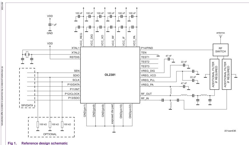
The purpose of components used in this schematic is described in <u>Table 1</u>. All parts marked with a star \* are UHF relevant materials and should be chosen according for this purpose. Special attention should be given to self-resonant frequency (SRF) and quality factor Q.
