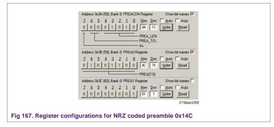
In this example, registers PREA2 and PRE3 are not configured because they are not relevant for the application due to the shorter preamble.
