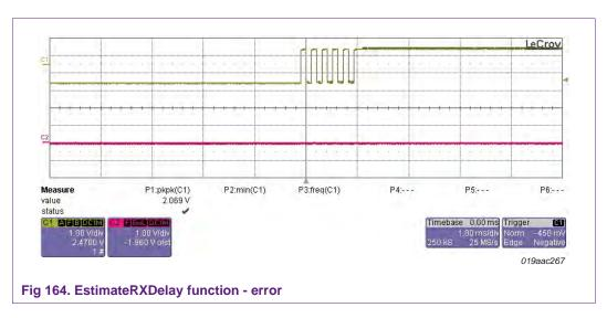
The OL2381 #1 sends and receives the known message and calculates the time delay between them. The argument is 3686500 / chip rate. 3686500 is half the microcontroller internal clock oscillator frequency and in our example the chip rate is 9600. MRXD (384) returns a chip delay of 787.
