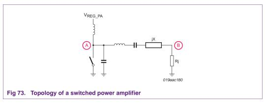
The switched PA can achieve a high efficiency because the current and the voltage of the transistor are switched at different moments as shown at point A of <u>Figure 74</u>. The output voltage of the class E amplifier is shown at point B of <u>Figure 74</u>.
