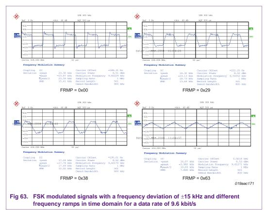
The effect of register FRMP on the signal is obvious. The higher the value of FRMP, the closer the signal resembles a triangular signal. The value of the frequency ramp should not be too high otherwise the ramp is slower than the data rate and frequency demodulation is impossible.
