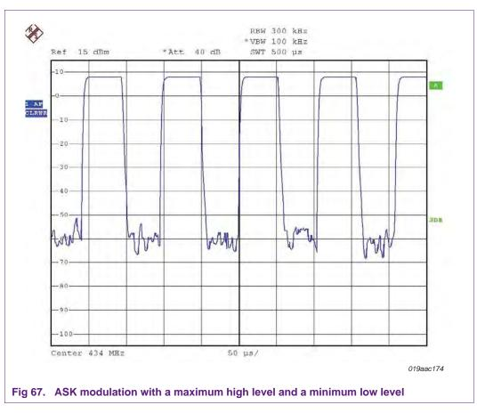
No amplitude ramping is performed in this section.
