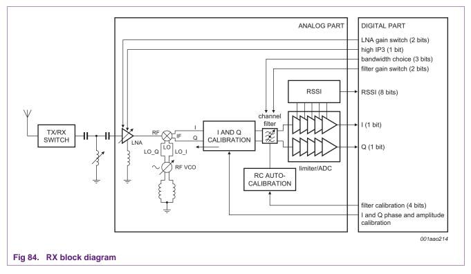
The OL2381 analog RF receiver front-end consists of LNA, mixer, channel filter and limiter.
