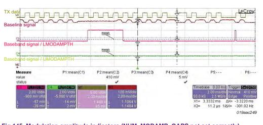
Fig 145. Modulation amplitude indicators (NUM\_MODAMP\_GAPS not set correctly)
