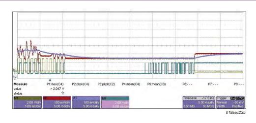
Fig 131. Baseband filter output, slicer threshold, and slicer output for long "1" sequence
