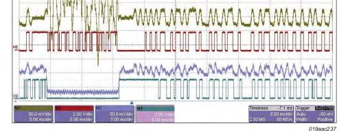
Fig 133. Baseband filter output and slicer output: interferer with the same power present
