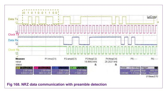
Data is received (blue trace) only when the receiver recognizes a valid preamble pattern. Otherwise, the receiver enters predefine mode (stop or power-down).
