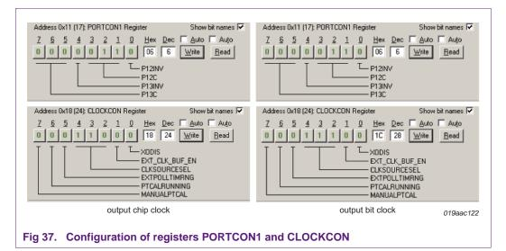
The value of CLKSOURCESEL does not have any influence on the data generation in transmit mode or data reception in receive mode.
