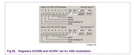
Flag F of transmit command (Figure 50 on page 43) determines if registers ACON0 or ACON1 are used in the ASK mode for the high level. If bit F = logic 0, register ACON0 is taken as the high level. If bit F = logic 1, the register ACON1 is taken as the high level. In both cases the register ACON2 is considered as the low level.
