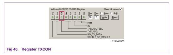
In normal use situations, the chip clock is set as the TX clock when NRZ encoding is used and the bit clock is set as the TX clock when Manchester encoding is used, as shown in <u>Table 16</u>. Further details of the chip rate calculation are given in <u>Section 5.4 on page 30</u>.
