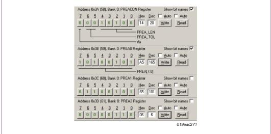
Fig 169. Register configurations for Manchester encoded preamble 0x14C
