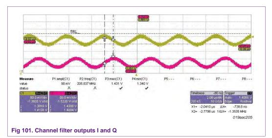
The bandwidth of the channel filter should be chosen carefully. In order to achieve the best signal-to-noise performance of the receiver it should be as close as possible to the bandwidth occupied by the modulated receive signal. If the bandwidth is chosen too wide, a large amount of noise is passed through the filter reducing the signal-to-noise ratio of the receiver. If the bandwidth is set too narrow, some data will be missed degrading the bit error rate measurement (receiver sensitivity).
