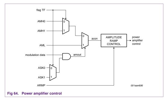
Registers ACON0 to ACON2 control the output amplitude and ASK modulation characteristics of the power amplifier. The lower 5 bits of control registers ACON0 and ACON1 allow two different high levels to be set (AMH0 and AMH1) and one low level (AML) in register ACON2. They define the modulation depth during amplitude modulation of the RF carrier. Bit 7 of ACON0 or ACON1 is set to logic 1 (shown in Figure 65) in order to activate the ASK modulation.
