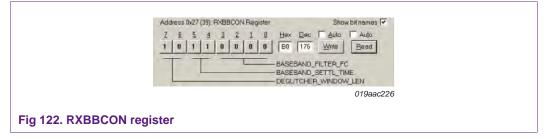
The baseband filter cut-off frequencies for various BASEBAND\_FILTER\_FC bit settings can be set in the range 221 Hz to 115.45 kHz; please refer to the OL2381 data sheet.
