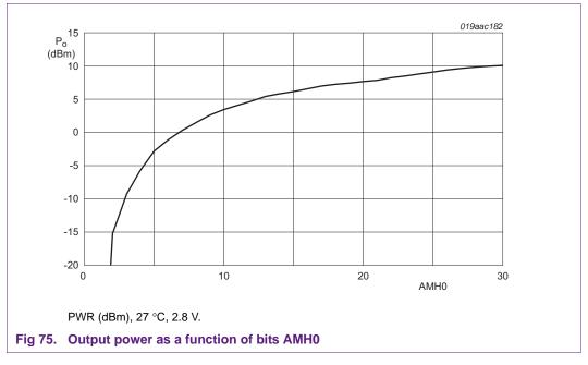
When the register AMH0 is close to 0x20, it corresponds to a major transition of the DAC. When it is in the region between 0x02 and 0x10, the PA is equivalent to a current source because the switch does not behave as a switch. If output power between -5 dBm and 0 dBm is needed, another matching topology should be used.
