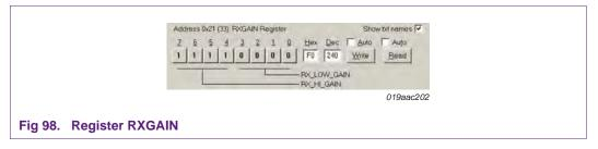
Bits 6 and 7 in register RXGAIN set the LNA value to "high gain mode", and bits 3 and 2 set the LNA value to "low gain mode". By setting bits 6 and 7 (or 2 and 3) four different gain settings (4 dB to 25 dB) can be chosen as explained in the OL2381 data sheet.
