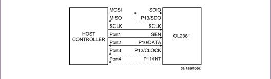
Fig 14. OL2381 Configuration for port communication
