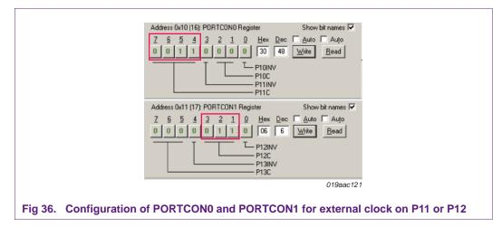
A bit or chip clock signal can be observed with an oscilloscope connected to pin P12 if register PORTCON1 is configured as output clock from clock generation according to the settings of CLKSOURCESEL (Figure 37). This is shown in Figure 38.
