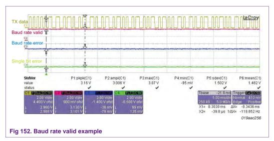
Figure 153 shows that the NRZ signal timing verification unit is virtually unused because of the single-chip timeout of 3.5, a value which can be smaller in practice. This will cause a single bit timing error almost every time.
