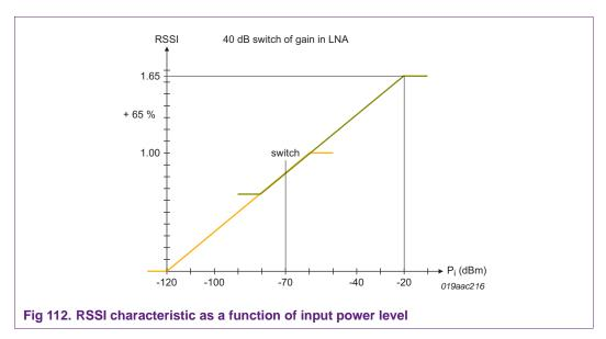
A compensation value can be set in register GAINSTEP (address. 0x23) as shown in Figure 113 in order to achieve a continuous RSSI reading when the gain setting of the front-end is changed. The register value is the difference in the RSSI readings (in the linear region) for the same input power between high and low gain mode. This value is added to the RSSI result when the low gain is activated. This seamlessly extends an overall dynamic range of the receiver to higher than 100 dB.
