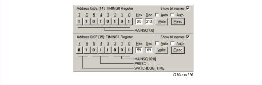
Registers TIMING0 (address: 0x0E) and TIMING1 (address: 0x0F) are set to 0xD5 and 0x59 for a baud rate of 9.6 kbit/s as shown in Figure 31.
