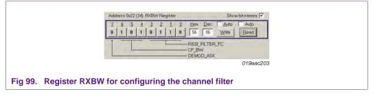
The configuration of the channel filter bandwidth (50 kHz to 300 kHz) is shown in the OL2381 data sheet.
