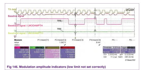
If the input sequence is Manchester encoded (has at least one transition between each two-chip interval) one gap has to be accepted and ignored.
