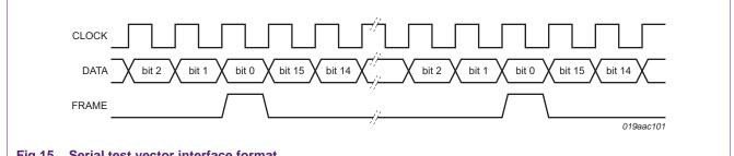
Fig 15. Serial test vector interface format
