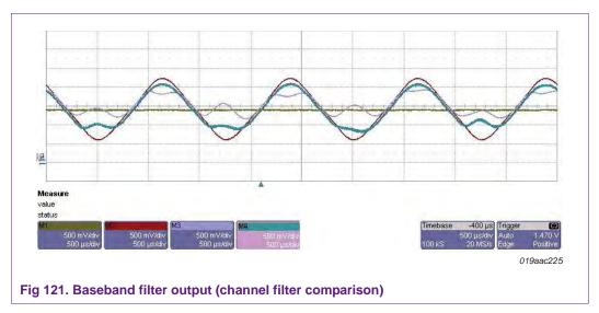
The red trace (triangle shape) is the DAC output (baseband filter output) with channel filter bandwidth set to 300 kHz.
