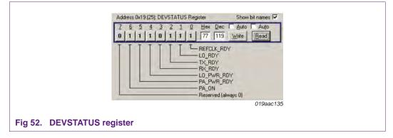
The different bits are explained in more detail in the OL2381 data sheet. Bits REFCLK\_RDY, LO\_RDY, TX\_RDY, LO\_PWR\_RDY, PA\_PWR\_RDY, and PA\_ON are set to logic 1 if TX mode is successfully activated, as shown in Figure 52.
