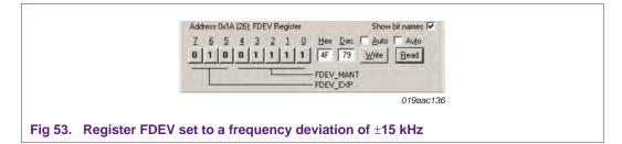
Setting the frequency deviation shifts the signal frequency.
