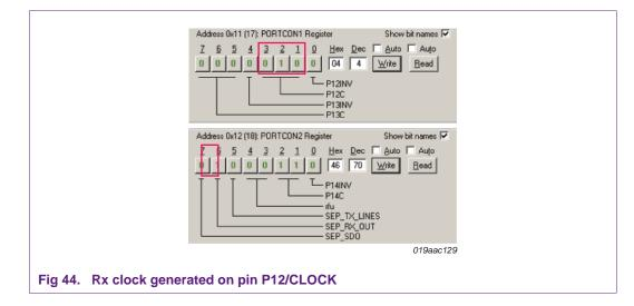
The clock is recovered from the received signal timing and informs the microcontroller when it is ready to sample data delivered at P10/DATA or SCLK.
