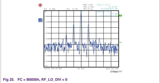
If the 14 LSBits of FC are interpreted as a signed integer, the modulation frequency of the disturber increases with the absolute value of this number. Due to the filter function of the PLL loop filter, the modulation index depends on the modulation frequency of the disturber. With the recommended setting of ICP = 2 the maximum modulation index is about 1 / 5, in other words the maximum power in the spurious emission is -20 dBc.
