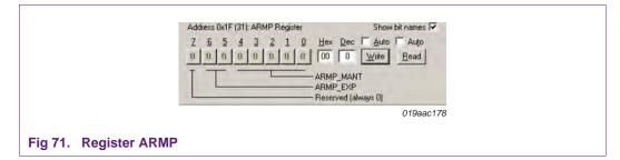
The ARMP register sets the number of 16 MHz clock cycles to be used to ramp the ASK amplitude from the lower AML value to the higher AMH value and vice versa. The number of clocks is calculated according to Equation 19.
